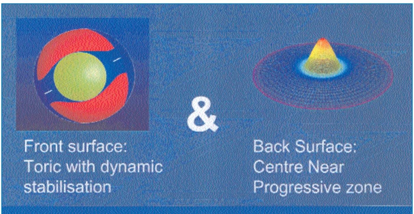
▼ Figure 2: CIBASOFT Progressive toric - soft progressive toric front and back surface design
