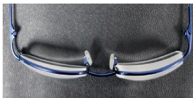
FIGURE 15. Both lenses are the same power – the lens on the left of the image is surfaced to a smaller diameter, the lens on the right glazed from a larger stock lens (note the nose pad splay angle).
