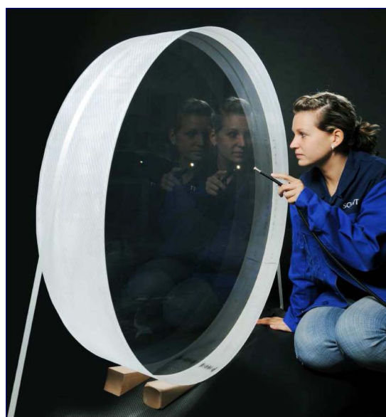
Fig. 13. (Color online) Large disk of the lead flint glass type LLF1 diameter 980 mm \times 210 mm, weight 0.47 tons (photo: SCHOTT).
