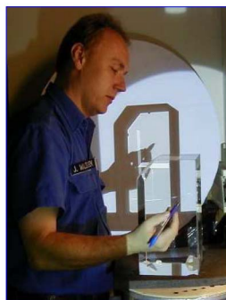
Fig. 19. (Color online) Shadowgraph setup for stria inspection. Right: application in practice. The main problem is to calibrate its results in relation to optics design via the wavefront distortion and structural width (photo: SCHOTT) [32].
