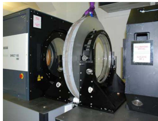
Fig. 16. (Color online) Homogeneity measurement of a 1 m diameter glass blank using a ZEISS DIRECT 100 interferometer at 500 nm aperture [25].
