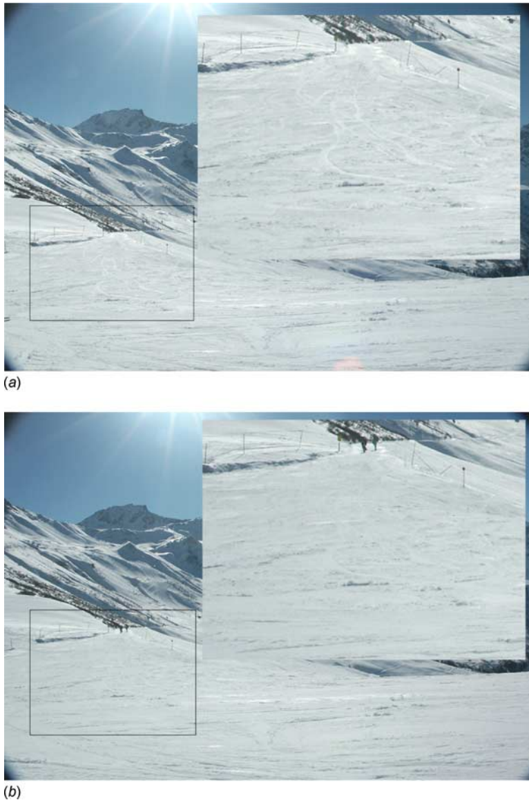
FIG. 6—(a) Direction of polarizer = 0^\circ . The lower left part is enlarged. All (glancing) traces are visible. (b) Direction of polarizer = 90^\circ . Most of the information is taken out! The traces nearly vanish with a skiing goggle with vertical polarization.
