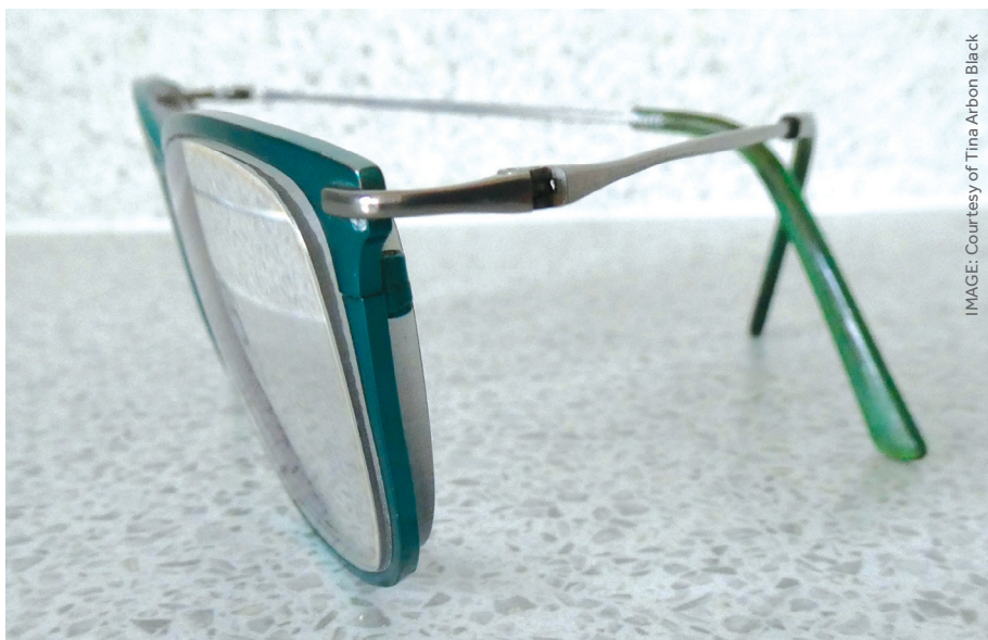
FIGURE 1. High minus spectacle lenses showing prominent edge thickness, minification and image displacement
